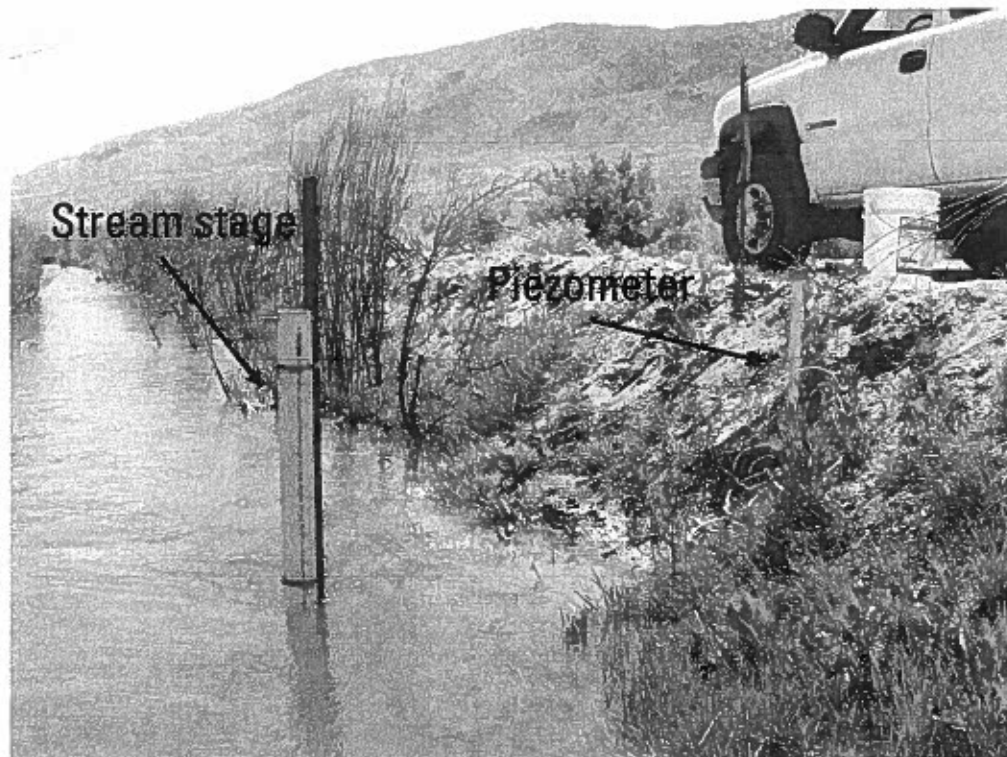
Figure 1. Photo from 5/6/2013 of stream (canal) stage and piezometer instrumentation at Canal 1A shortly after installation, Schurz, Nevada.
