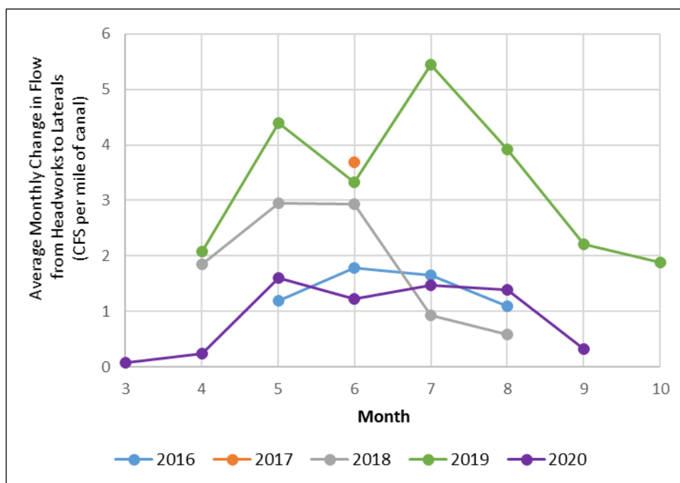
Figure 6. Monthly average change in flow (CFS per mile of canal) from the Saroni Headworks to Laterals A and B (based on monthly averages of available daily data)
